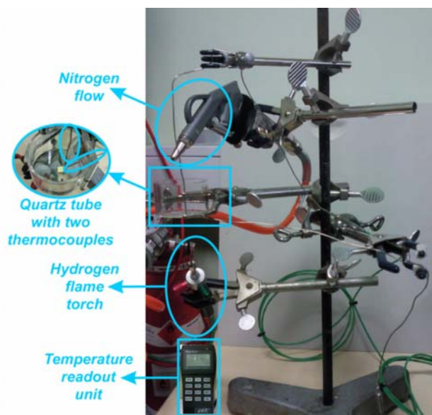
Figure 1: Image of the used experimental setup with explanation of the most crucial parts. Nitrogen and hydrogen cylinders are not shown on the image.
